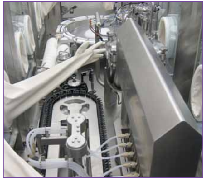
HPV can decontaminate complex work areas housing sensitive electronics.
