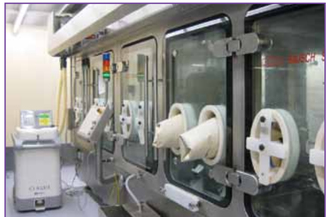
Bioquell Clarus® HPV generator hooked up to a large filling line.
